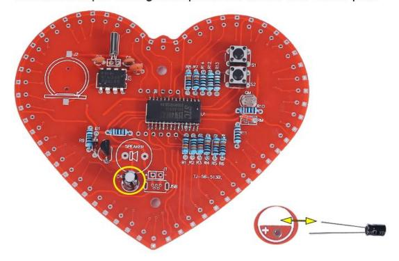
Step 17: Install 1pcs Passive buzzer at SPEAKER. Pay attention to the installation direction.
